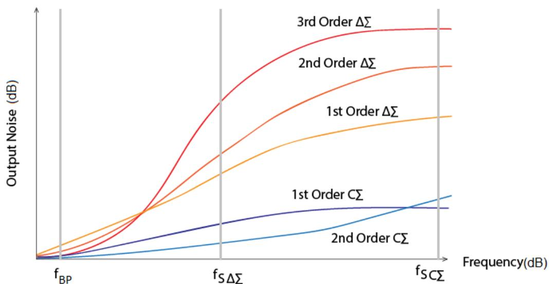
Figure 4: Relative noise floor shapes<sup>7</sup>
