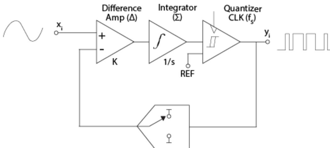
Figure 1: Delta-Sigma value to time domain converter.<sup>1</sup>
