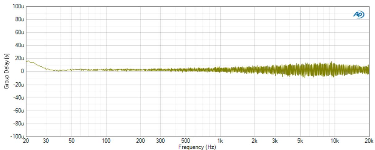
Figure 3: First order Continuous-Sigma exhibiting virtually zero group delay<sup>4</sup>.
