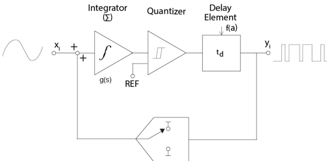
Figure 2: Continuous-Sigma value to time domain converter.
