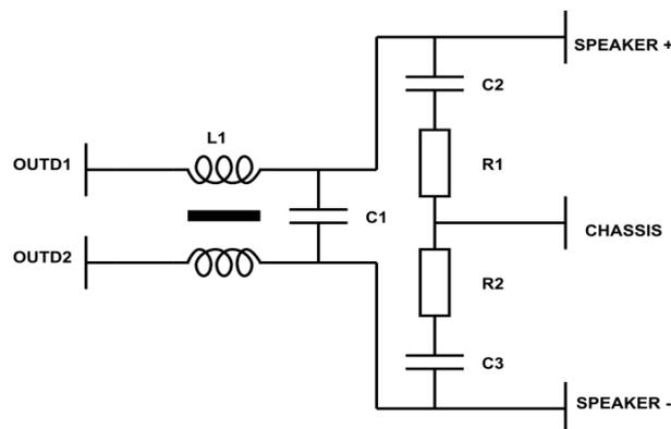
Figure 6: Simple, damped output filter<sup>10</sup>
