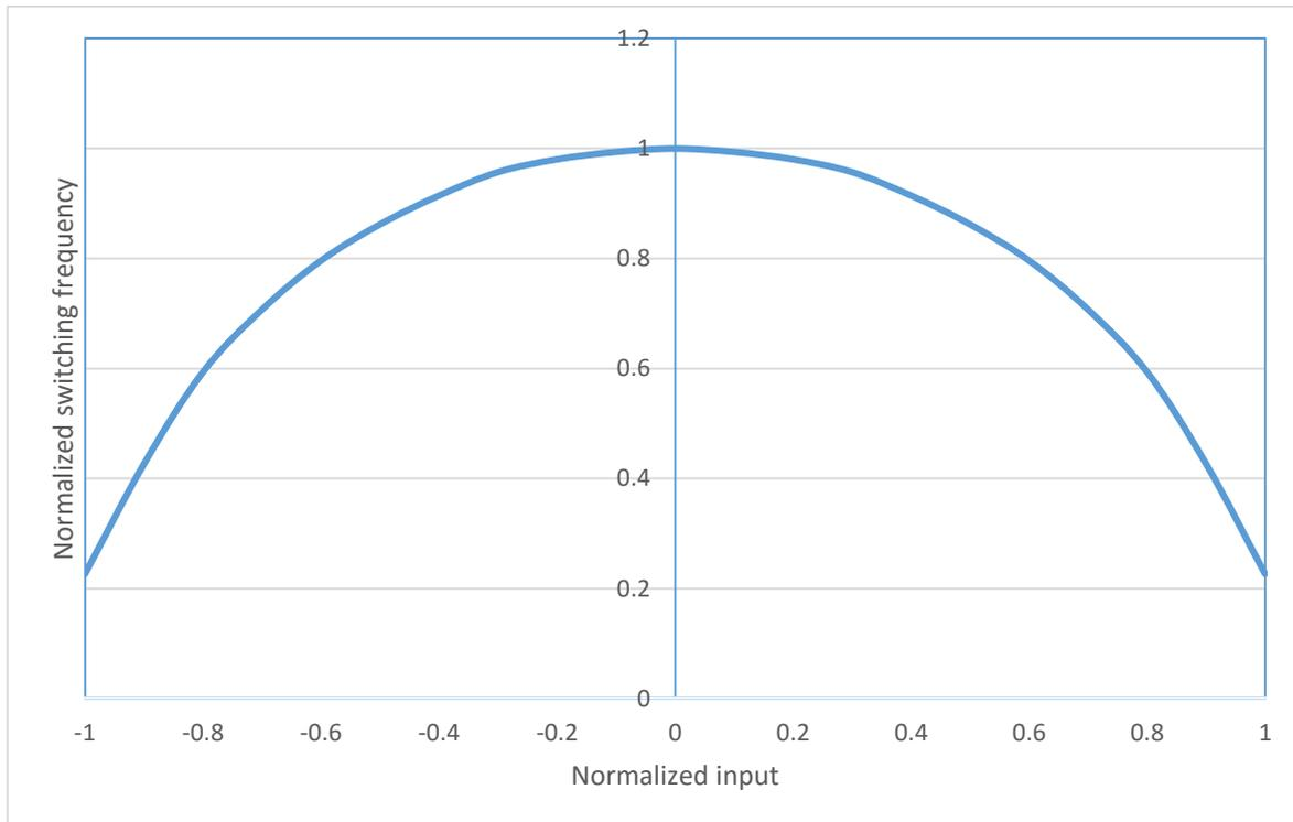
Figure 5: Switching frequency vs input signal
