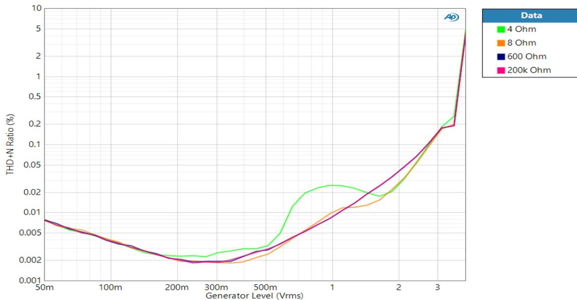
Figure 8: THD+N for 4Ω, 600Ω and 200KΩ load
